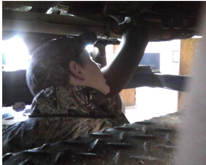
WADE HERRING AND SKYLER RICH INSTALLING A KNOCK SENSOR
